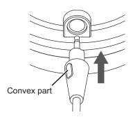
2 Rotate the convex part of the cable plug approximately 45 degrees clockwise to the position shown in the diagram to lock the cable plug.
