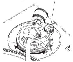
Refer to the following table to adjust the [**HEIGHT ADJUST**] dial to match the height to your cartridge size.
