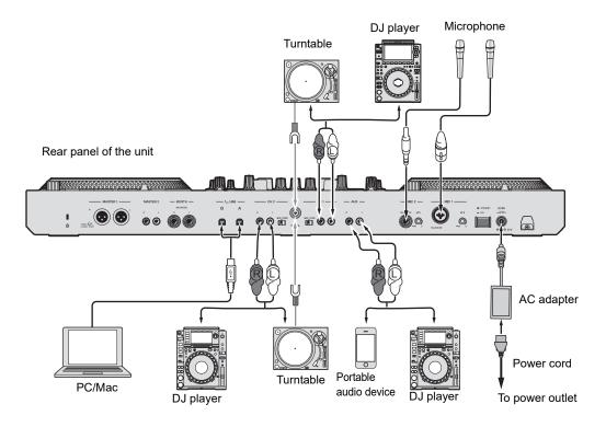
Set the [LINE/PHONO] selector switches for the [CH 1] and [CH 2] terminals to [PHONO]
