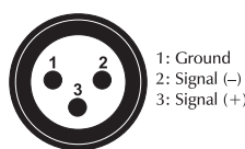
DMX-input XLR mounting-plug:
